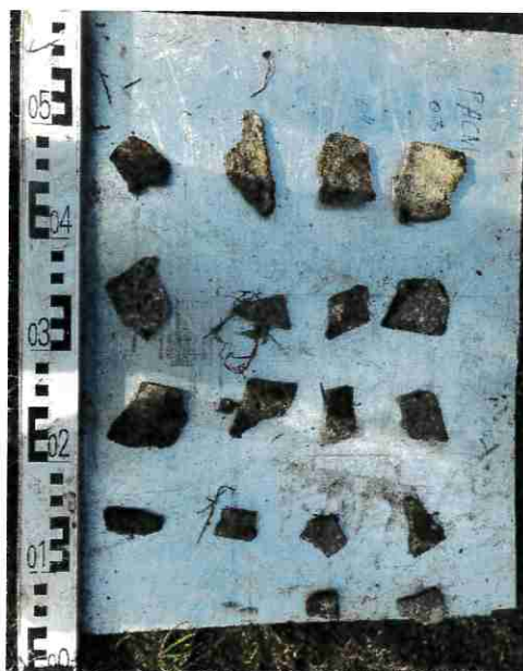
Figure 2, Confirmed Asbestos Cement fragments.
