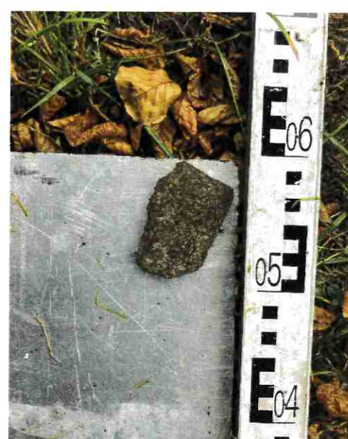
Figure 3, Confirmed Asbestos Cement fragment.
